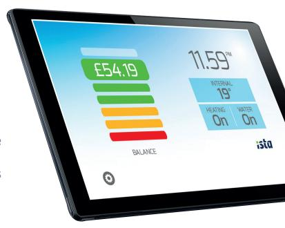
SmartPay combines industry leading smart meters and a world class billing system supporting online and retail terminal payment services. Using the latest in wireless M-Bus technology, data is collected from meters and automatically sent to ista's billing and reporting systems.
