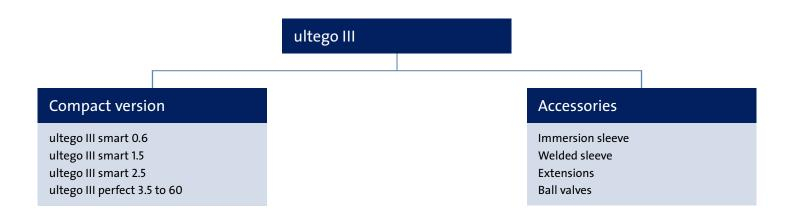
The ultego III ultrasound heat meter product range includes compact versions, combined heat meters and extensive accessories.
