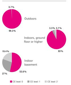
Figure 4: Distribution of CE levels outdoors, indoors above ground and indoors below ground level
