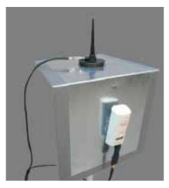
Figure 1: Measurement setup showing the scanner antenna (on top) and the housing containing the antenna feeding the Quectel BG96 module
